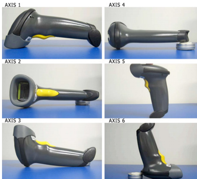
Figure 3. Hand-held barcode scanner dropped in 6 axes during shock testing.
