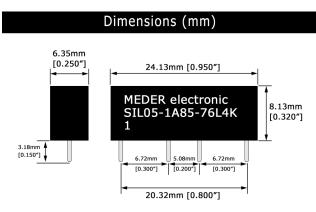
Figure 1. SIL HV Physical layout
