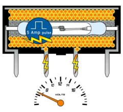
Figure 2. Depicts a perfect square wave pulse of 5 Amps traveling across the closed reed switch contact surface.
