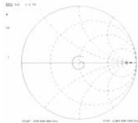
Fig. #25 Shows a Smith Chart plotted for frequencies to 4 GHz. The second dotted circle starting from the right is the 50 Ohm impedance point.
