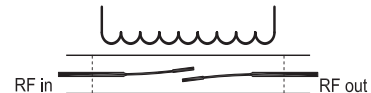
Fig. #3 A Reed Switch mounted internal to a coaxial shield provides and excellent RF path for Giga Hertz frequencies.
